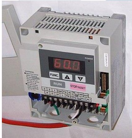
Variable Frequency Drivers (VFDs)
